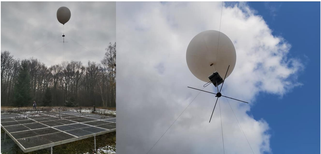
Figure 36: (left) Experiment carried out in December 2019 with the captive weather balloon above the 8m x 8m BRAMS transmitter in Dourbes. (right) The payload platform connected to the two short dipole antennas located below the helium-filled weather balloon. Three ropes are used to keep the balloon in its intended position.
